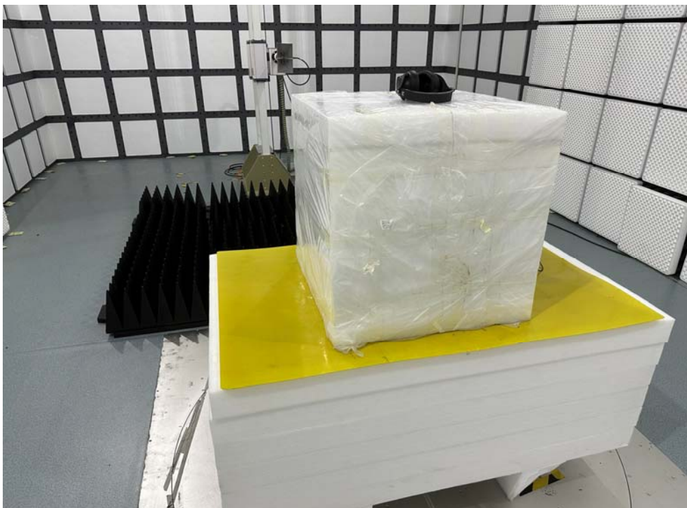
Photo of Radiated Emission Measurement (Above 1G)
