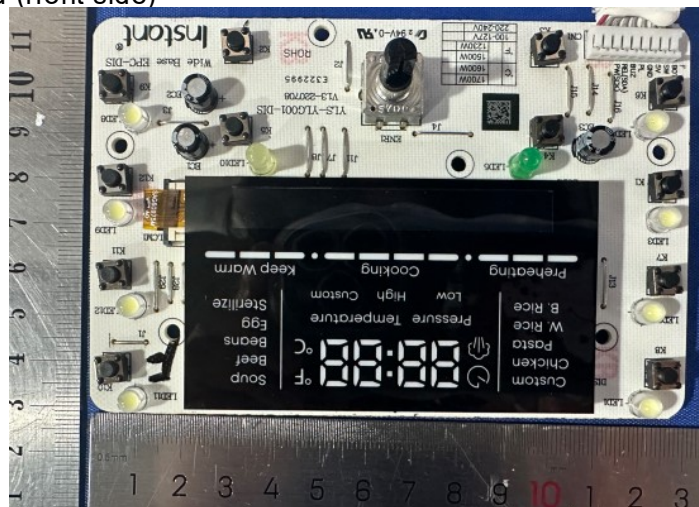
Photo 5 control board (front side)
