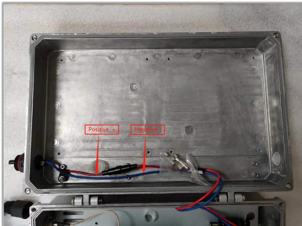
At the power interface (Power interface), connect the AC220V power cord. Note that the red line is the positive pole of the power supply, and the blue line is the negative pole of the power supply. Please do not connect it wrongly! !
