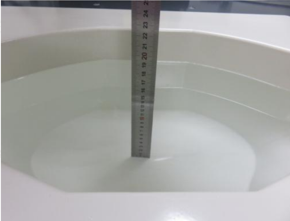
Photograph of the depth in the Body Phantom (1900MHz, 16.0cm depth)
