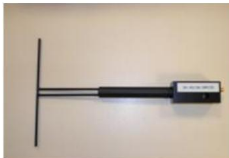
Figure 1 – Satimo COMOSAR Validation Dipole
