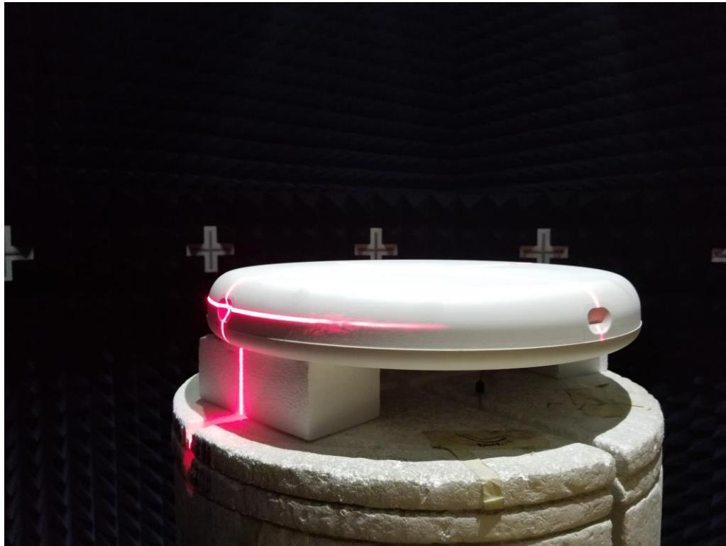
The EUT was placed on top of the Styrofoam mast in a holding fixture at the 0° position.
