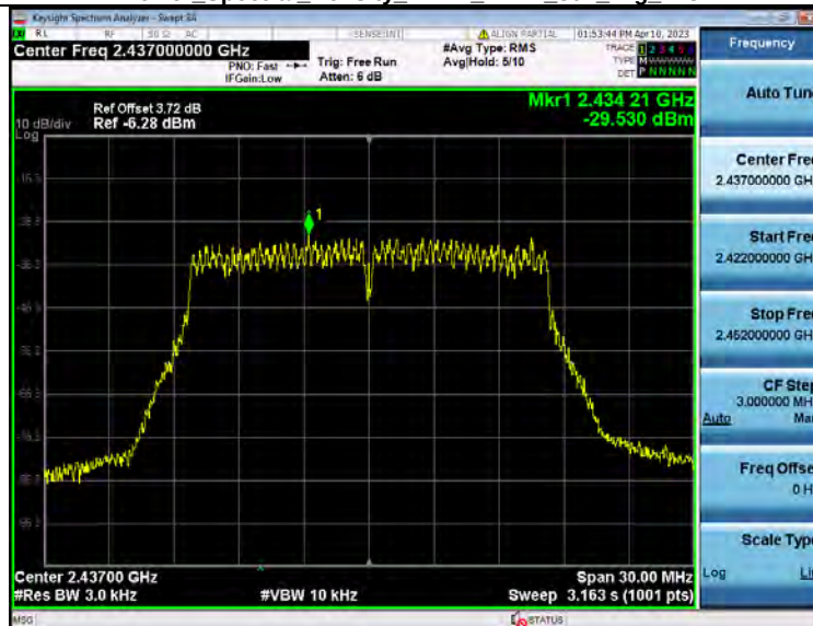
Power Spectral Density NVNT_ANT1_802_11g_2437
