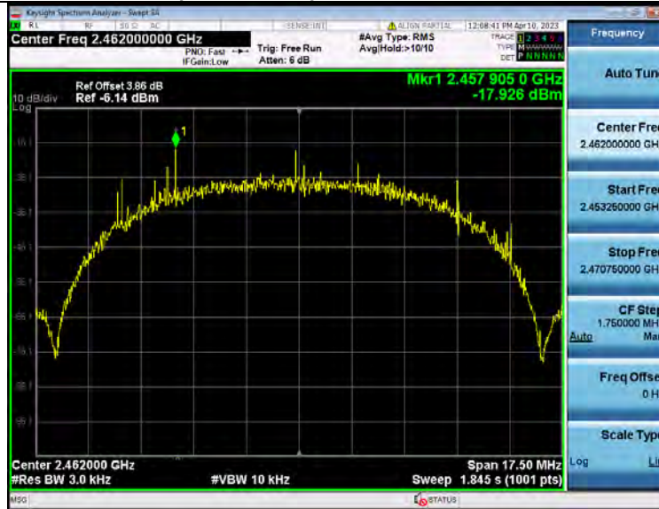
Power Spectral Density NVNT_ANT1_802_11b_2462
