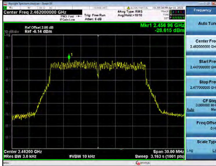
Power Spectral Density NVNT_ANT1_802_11g_2462
