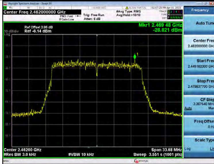
Power Spectral Density NVNT_ANT1_802_11n(HT20)_2462
