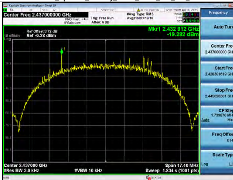
Power Spectral Density NVNT ANT1 802.11b 2437
