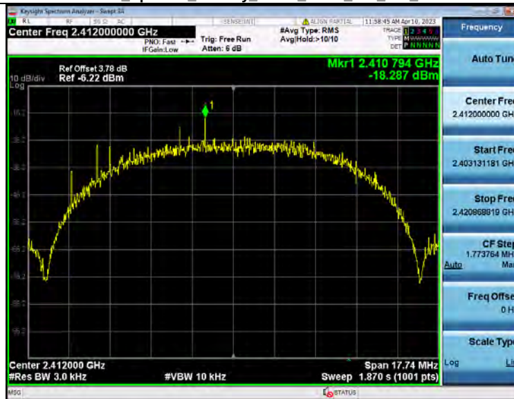
Power Spectral Density NVNT ANT1 802.11b 2412
