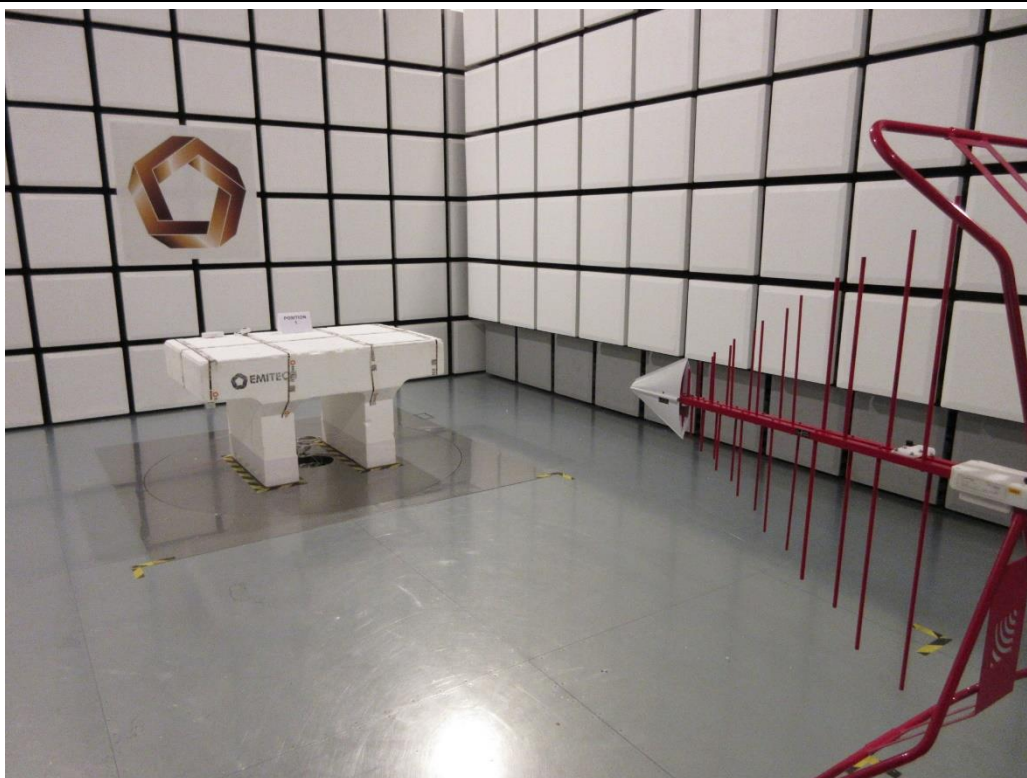
TEST SETUP PHOTO(S) - RADIATED MEASUREMENT – 30MHZ TO 1GHz
