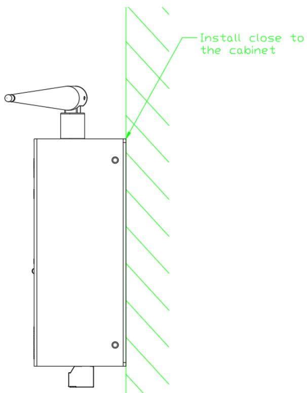
During installation, first attach the gateway to the backplane of the cabinet, and then fix it with screws. The control cabinet with good tightness and convenient subsequent wiring arrangements should be used. The control cabinet should be placed in an open, dry and non-corrosive liquid place to avoid damaging the equipment.
