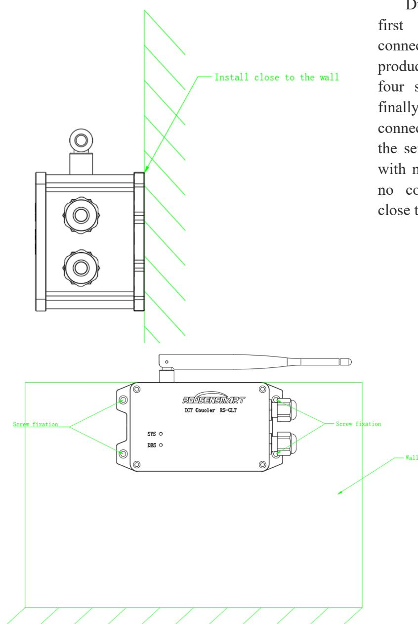
During installation, first remove the PG connector, then attach the product to the wall, fix the four screws in turn, and finally reconnect the PG connector. When installing the sensor, choose a place with no obvious shielding, no corrosive liquid, and close to the sensor.
