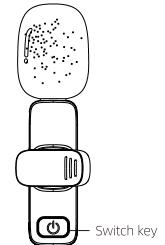
Step 2: Press switch key of microphone, the indicator light turns green, and then power is turned on.
