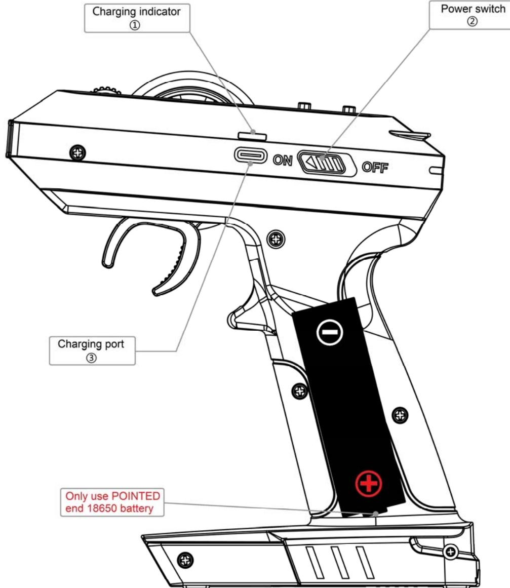
■ **Installing battery** : remove the battery door from the bottom of the transmitter, install battery as shown. ONLY use Li-ion or Li-pol POINTED end 18650 battery, charging voltage 4.2V maximum.
