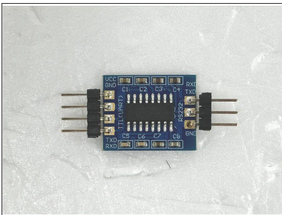
**Top view of Sub2 PCB**
