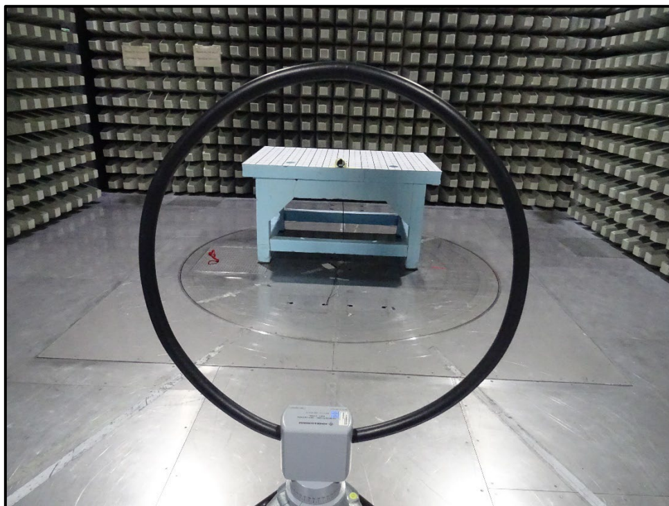
Picture 1 Radiated Test Setup-9 kHz to 30 MHz
