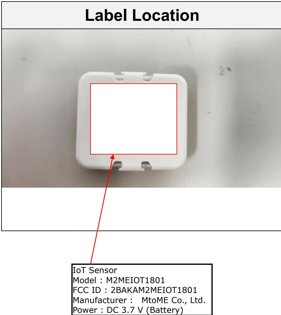
The device is so small that it is not practicable to place the statement specified under 15.19 statement request, the information required by this paragraph shall be placed in a prominent location in the User's Manual.
