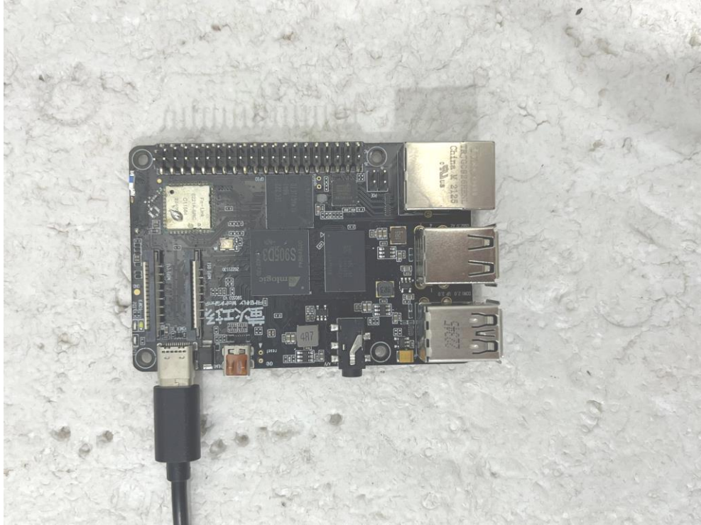
12.2.Photo of Conducted Emission test
