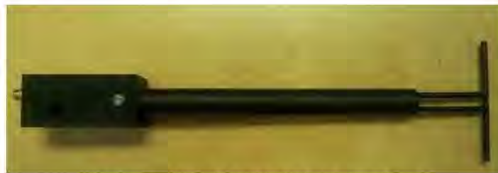
Figure 1 – MVG COMOSAR Validation Dipole
