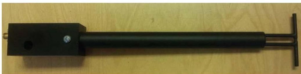
Figure 1 – MVG COMOSAR Validation Dipole
