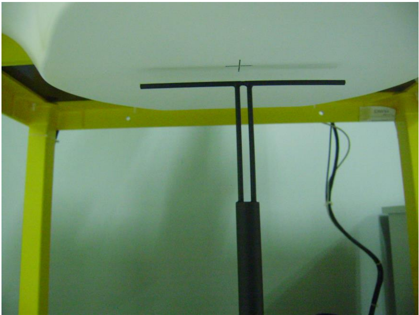
Setup Photo of Dipole Antenna
