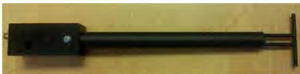
Figure 1 – MVG COMOSAR Validation Dipole
