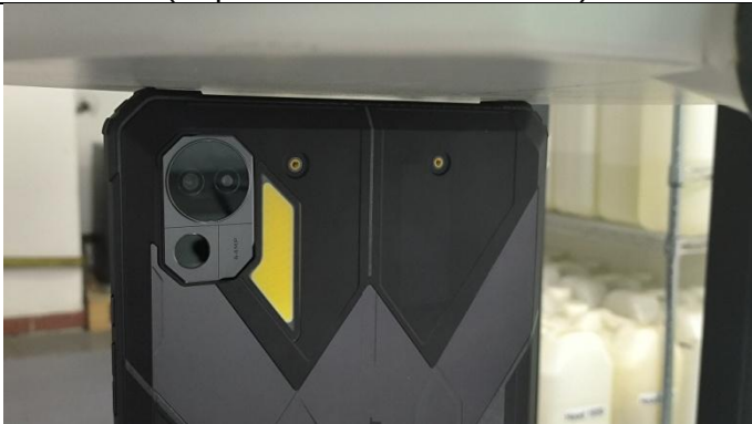
Top Side (Separation distance of 0mm)
