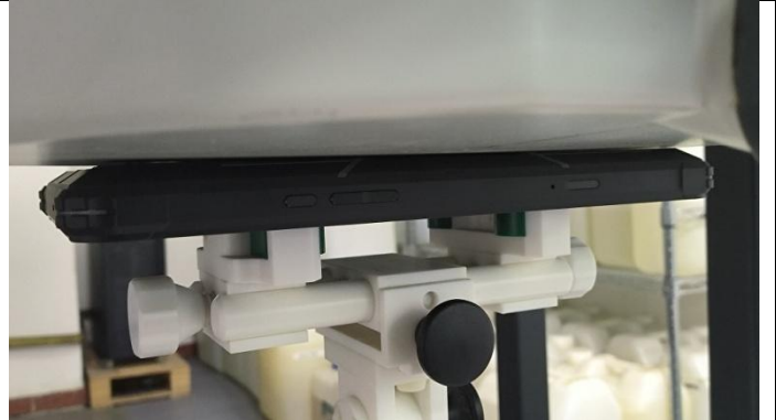
Right Side (Separation distance of 0mm)
