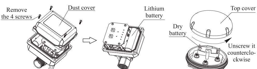
Remove the 4 screws on the dust cover, remove the old lithium battery, replace it with a new one, and insert the plug.
