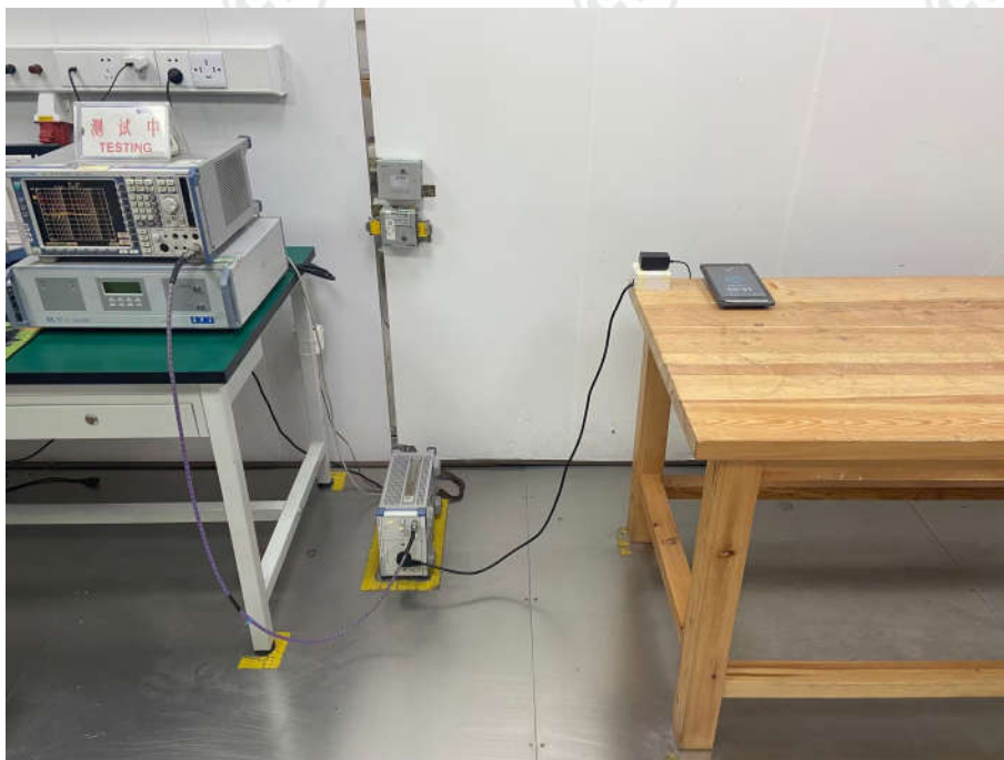
Conducted Emissions Test Setup
