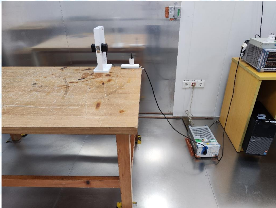
Photo of Setup for Conducted Emission
