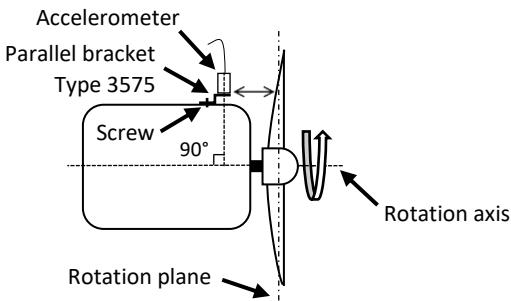
⚠ • **Screw the accelerometer to the bracket and secure it with the appropriate amount of torque on the platform**
