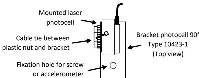
➤ The photocell bracket can be secured using an accelerometer to reduce the installation overall size. It is also possible to use screws to mount the photocell by itself
