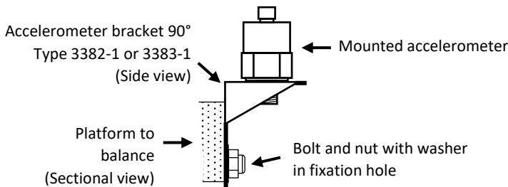
⚠ • **Connect the cable to the accelerometer by screwing it by hand and secure the cable with cable ties or with an adhesive**
