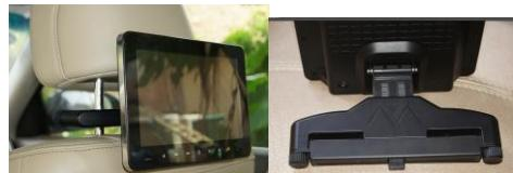
2. Remove the screws from bracket like below picture .
