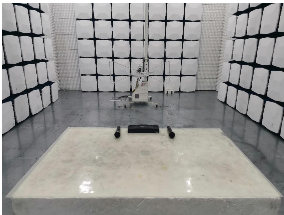
Photo of Radiation Emission Test
