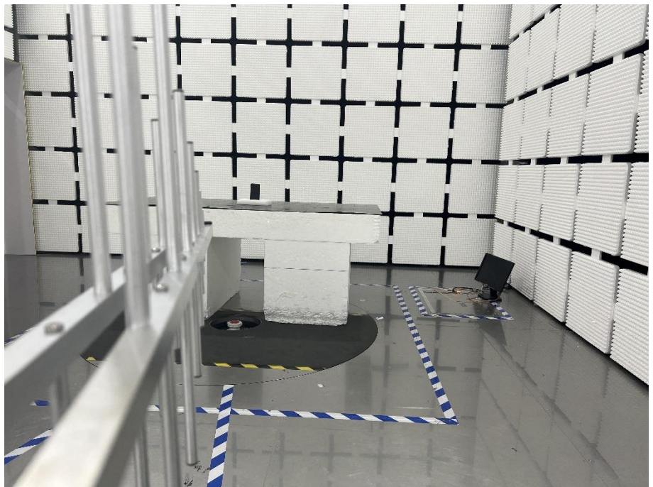
Radiation Emission Test Setup (30MHz to1GHz)
