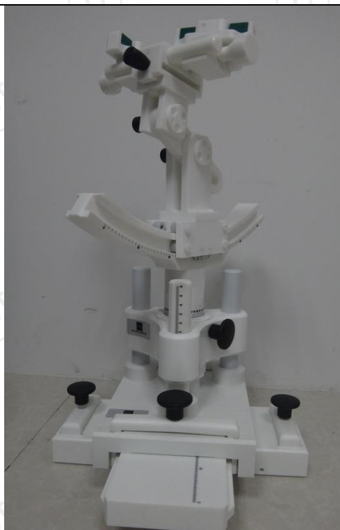
COMOSAR Mobile phone positioning system
