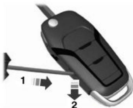
1. Insert a screwdriver, in the position shown and gently push the clip.
