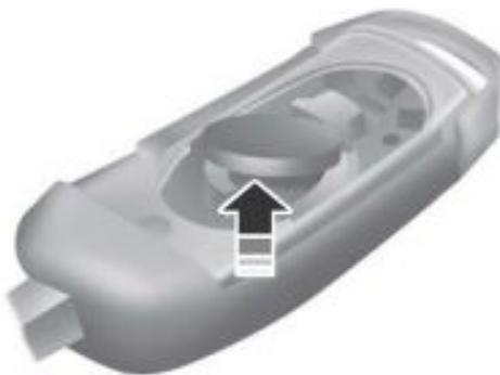
**Note:** Do not touch the battery contacts or the printed circuit board with the screwdriver.
