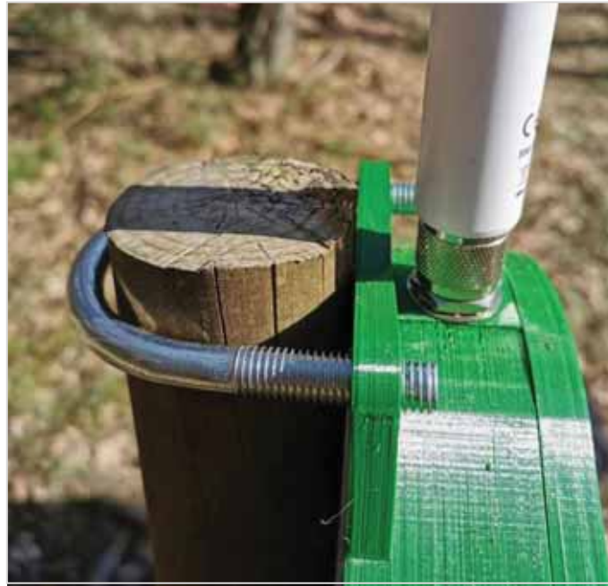
Arrange clamps around pole
