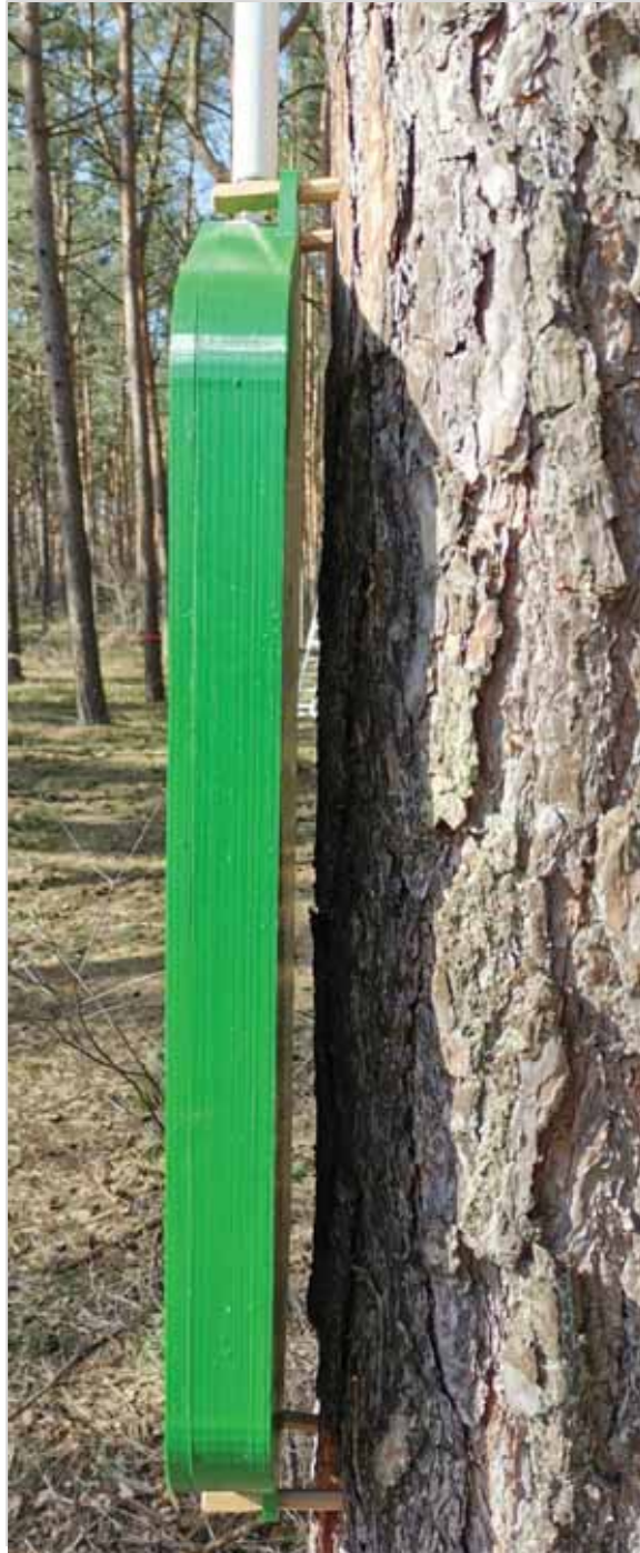
Mesh Gateway deployed and 2 cm away from the tree
