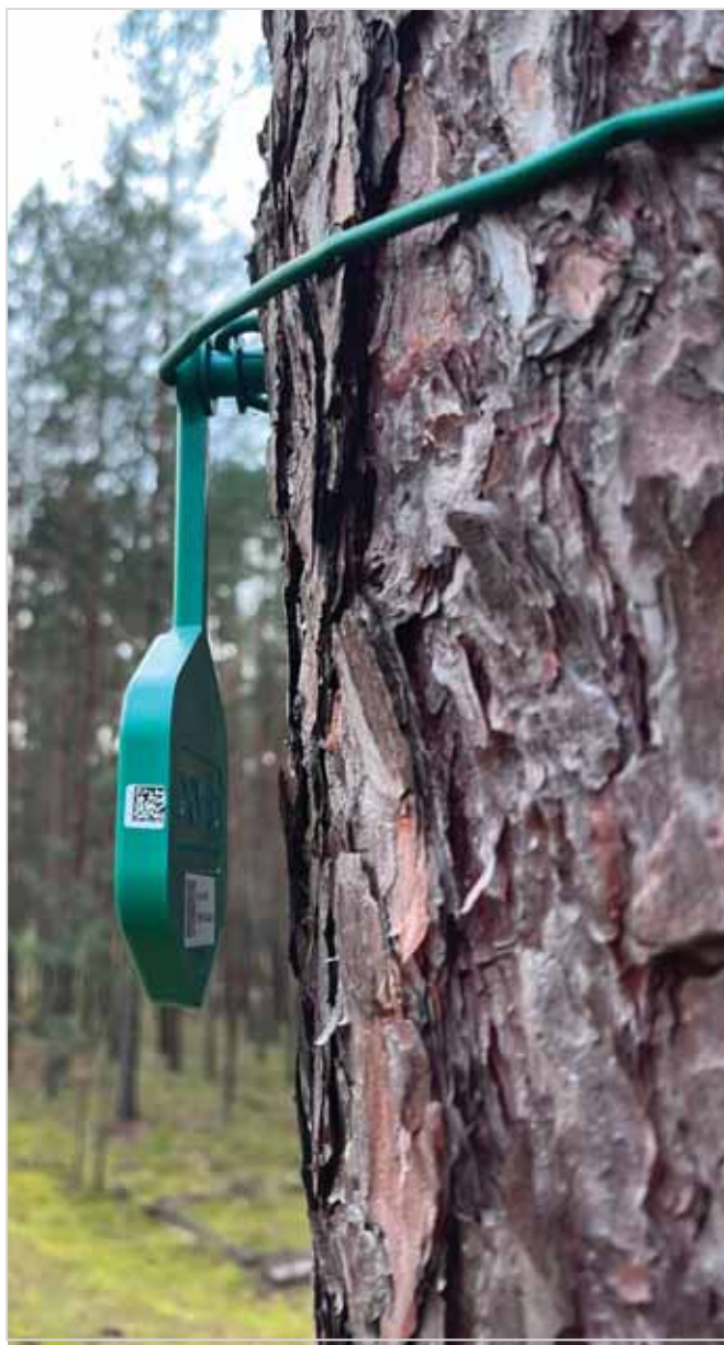
Sensor attached with crop wire
