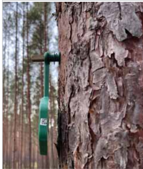
Attached sensor using tree nail
