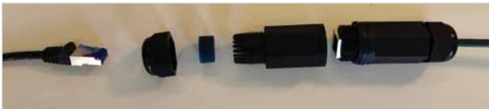
Border Gateway disassemble Ethernet connector
