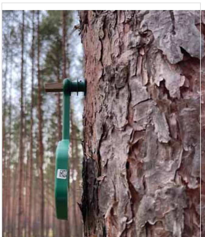
Sensor attached with treenail and spacer
