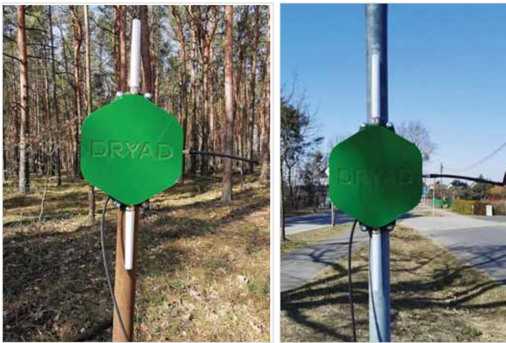
Border Gateway deployed on a pole
