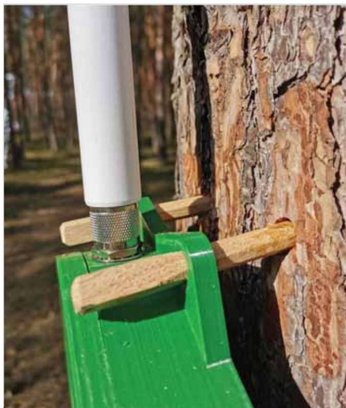
Mesh Gateway attached at the top
