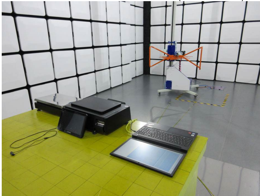
RADIATED RF MEASUREMENT SETUP (30MHz ~ 1 GHz)
