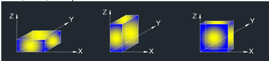
Note: The EUT uses an adjustable antenna, the antenna can be adjusted from 0° to 90°, all the typical positions have been explored, the 90° was the worst case, so the EUT in one orthogonal axis (X axis) emissions with 90° of the antenna has been tested and recorded in the report for all radiated test.
