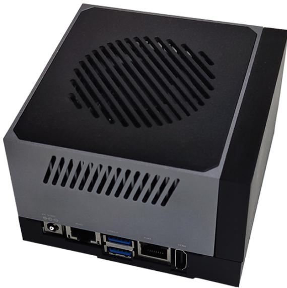
GEKit Orin is an embedded artificial intelligence computer independently designed and developed by Leetop based on Nvidia AGX Orin module, which can give computing power up to 200/275 Tops to many terminal devices.
