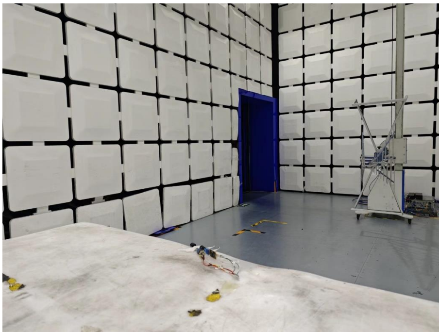
Description: Radiated Emission Test Setup for 30MHz ~ 1GHz (Mode1)
