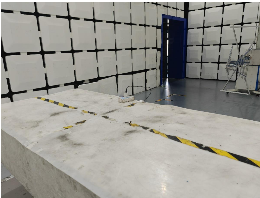
Description: Radiated Emission Test Setup for 30MHz ~ 1GHz (Mode1,2,3)
