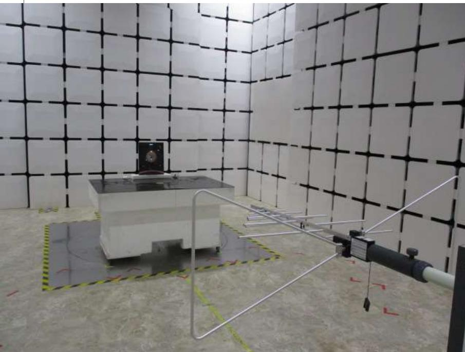
A photograph of a radiated measurement setup in an anechoic chamber. The setup includes a white rectangular test fixture on a grey floor, a black rectangular device on top of it, and a large black rectangular antenna mounted on a silver tripod. The chamber walls are covered with a grid of black absorbers. A yellow and black caution tape marks the measurement area on the floor.                                                                                        |
