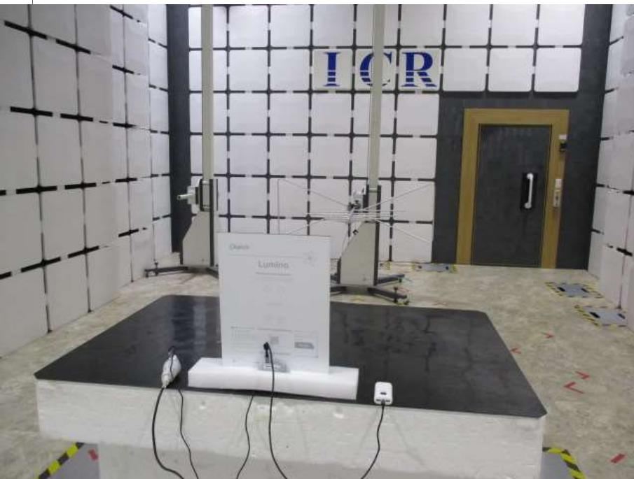
A photograph of a radiated measurement setup in an anechoic chamber, viewed from the rear. The setup includes a white rectangular test fixture on a grey floor, a black rectangular device on top of it, and a large black rectangular antenna mounted on a silver tripod. The chamber walls are covered with a grid of black absorbers. A blue banner with the text 'ICR' is visible in the background. A yellow and black caution tape marks the measurement area on the floor. |
