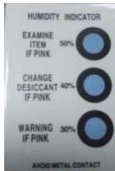
Figure 4-2 Temperature and humidity indicator CARDS
