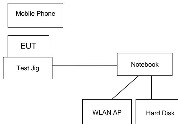
This example is connection diagram of EUT test configurations.
