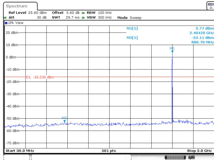
**Conducted Spurious Emission Plot on Bluetooth LE 2Mbps****GFSK Channel 00**
