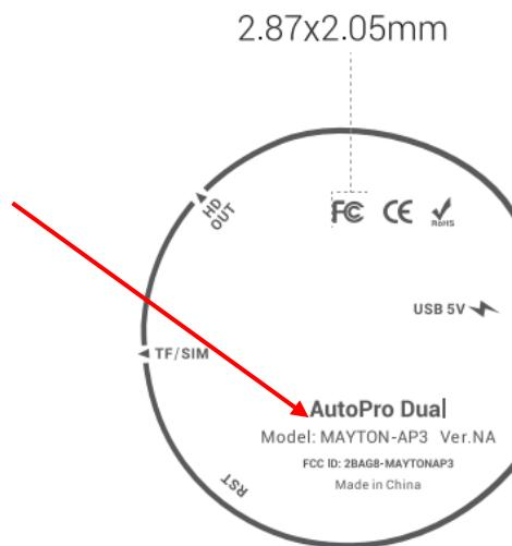
The label shown shall be permanently affixed at a conspicuous location on the device and be readily visible to the time purchase (Labeling requirements per 2.295)
