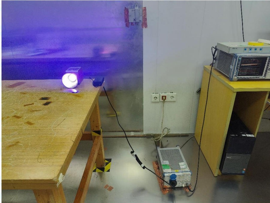
Photo of Setup for Radiated Emission (30MHz~1GHz)
