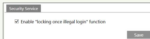
In order to prevent against malicious password unlocking, “locking once illegal login” function can be enabled here. If this function is enabled, login failure after trying six times will make the login interface locked. The camera can be logged in again after a half hour or after the camera reboots.
