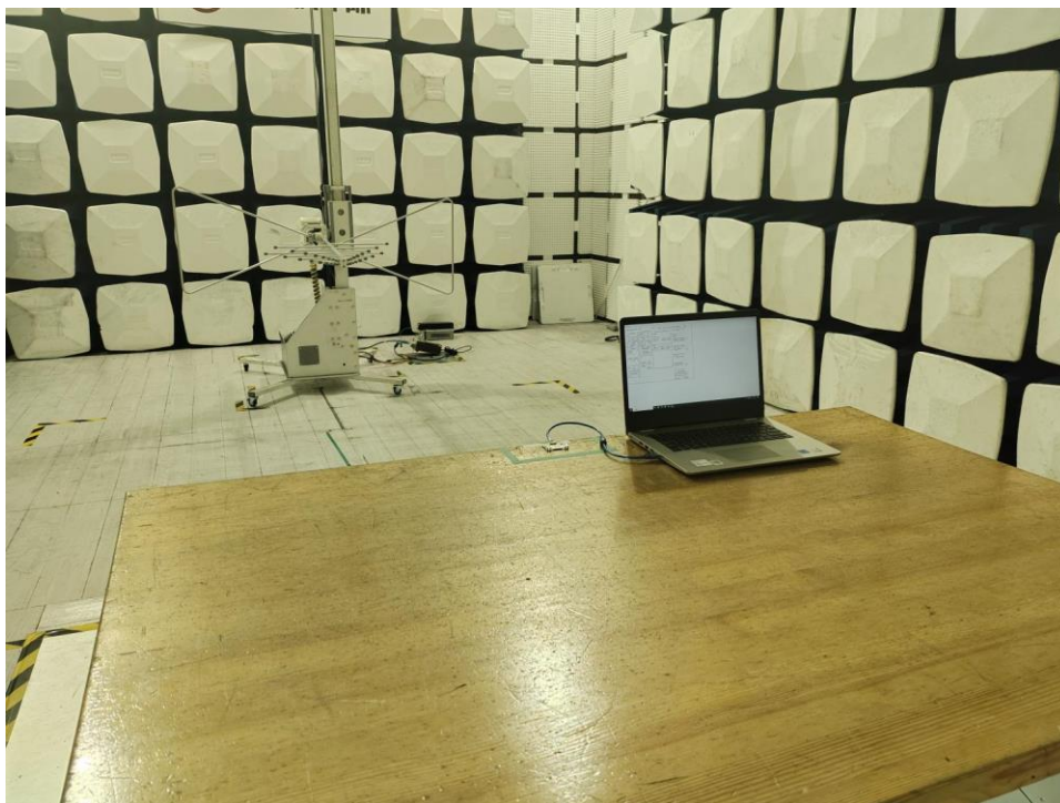
Photograph 1: Set-up for Radiated Spurious Emission, Below 1GHz
