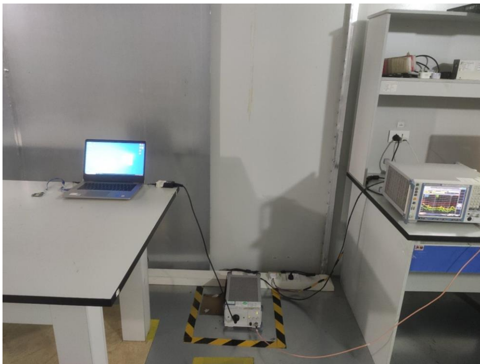
Photograph 3: Set-up for Conducted Emission on AC Mains
