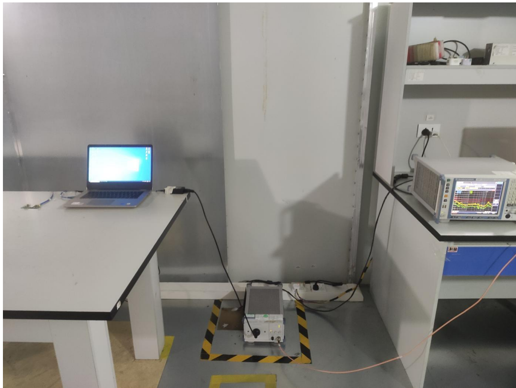
Photograph 3: Set-up for Conducted Emission on AC Mains
