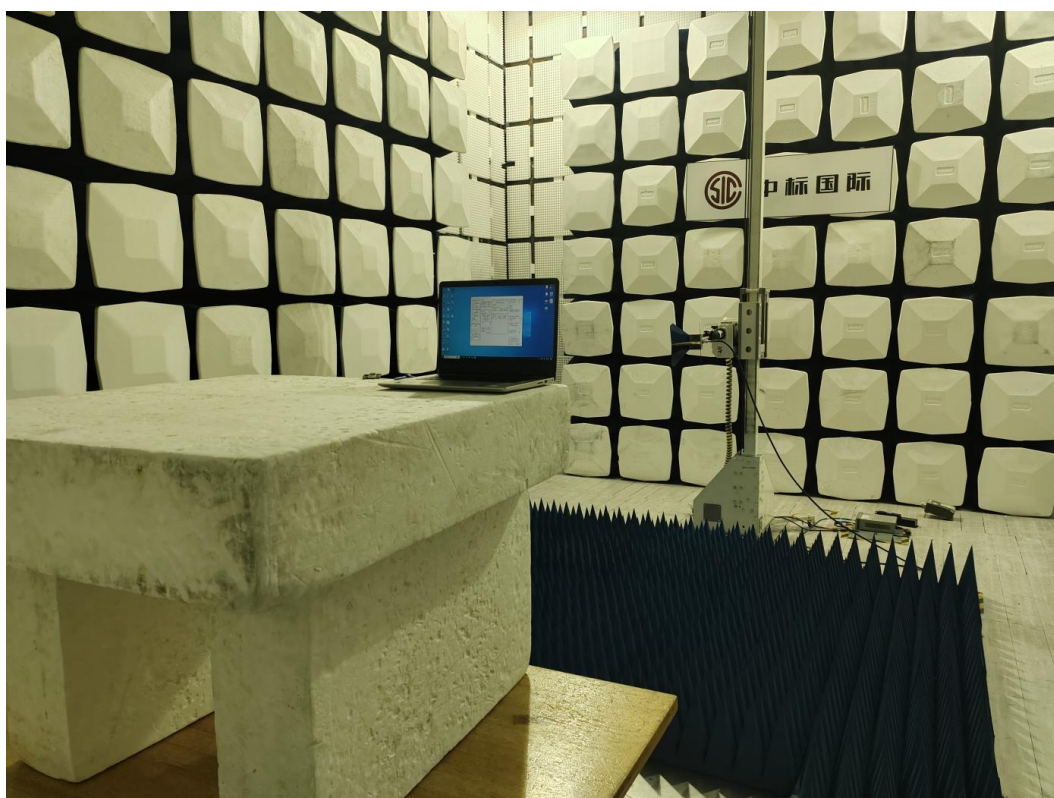
Photograph 2: Set-up for Radiated Spurious Emission, Above 1GHz
