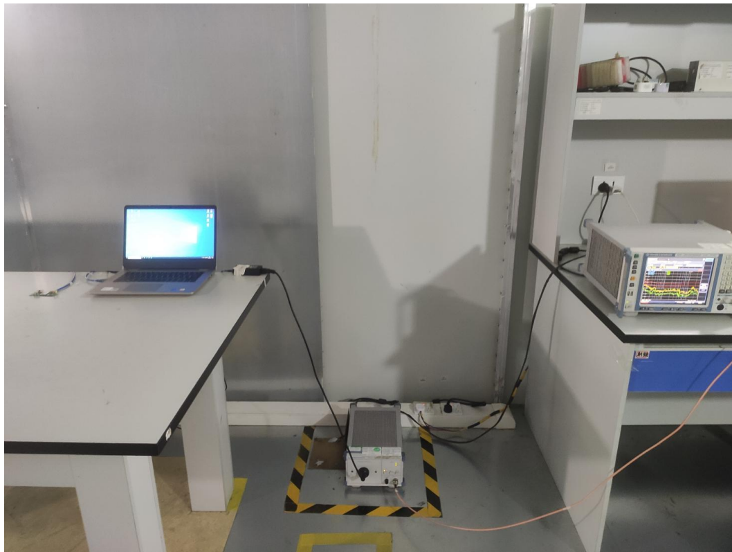
Photograph 3: Set-up for Conducted Emission on AC Mains
