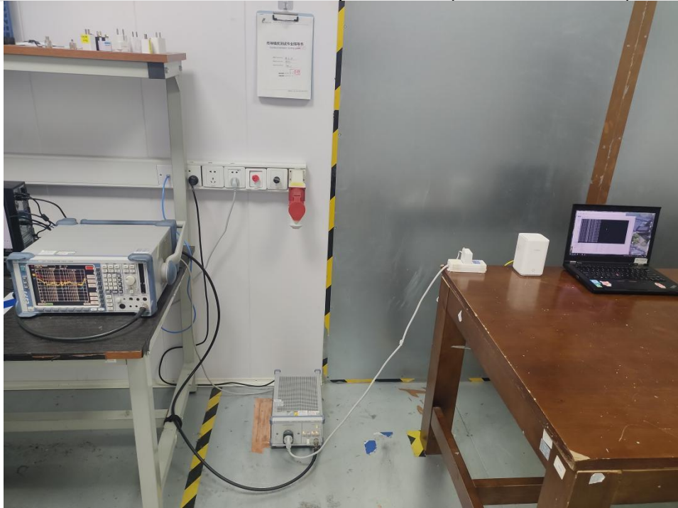
Conducted emissions at AC power line (150 kHz-30 MHz)
