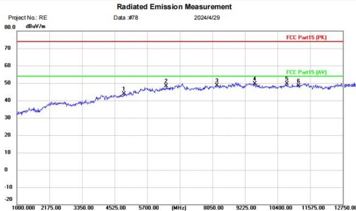
Site Polarization: **Vertical** Temperature: (C)
