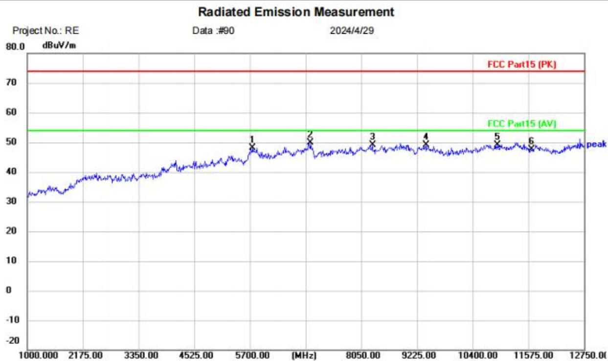
Site Polarization: **Vertical** Temperature: (C)
