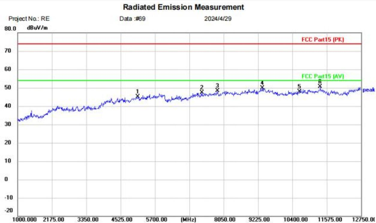
Site: Limit: FCC Part15 (PK) Polarization: **Horizontal** Temperature: (C)
