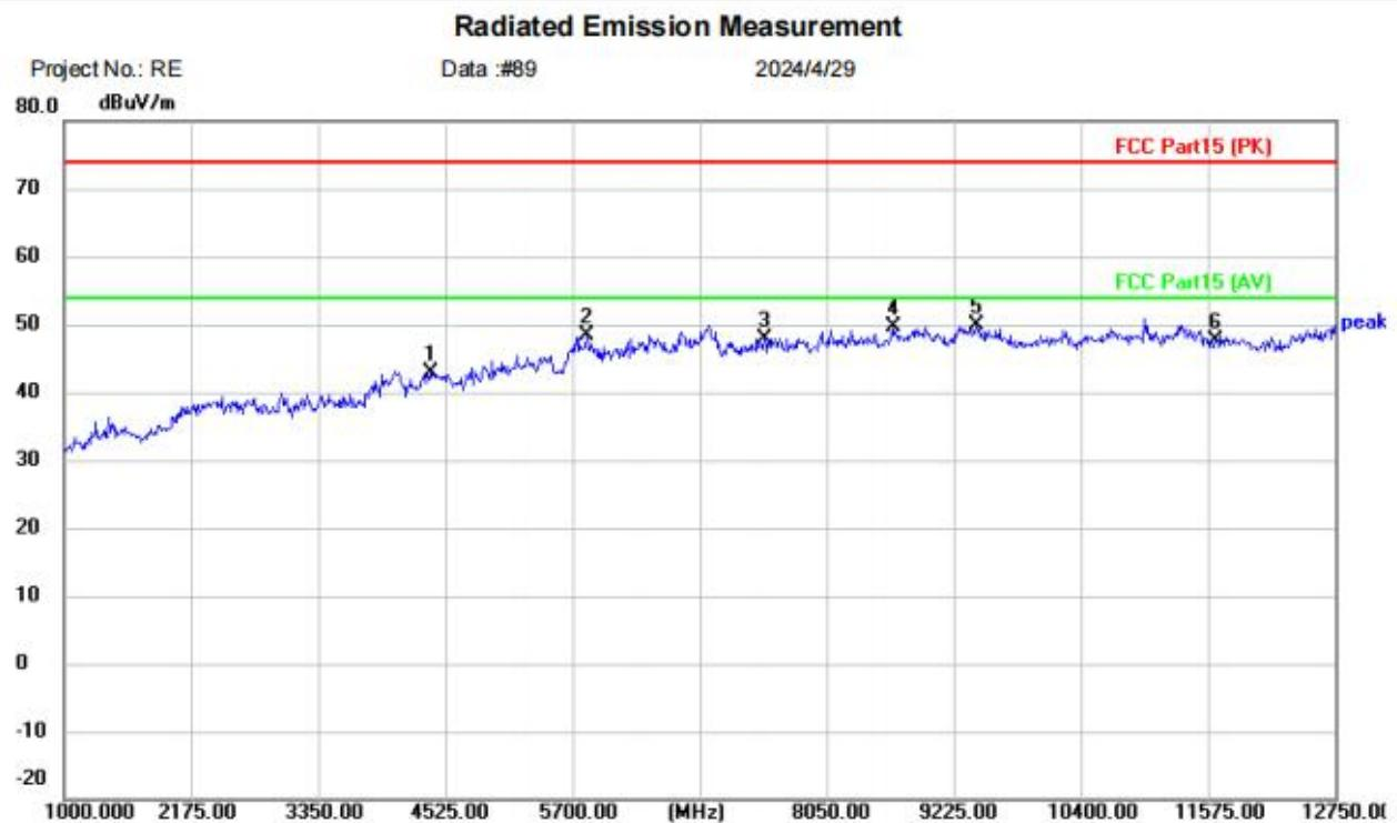
Site Polarization: **Horizontal** Temperature: (C)
