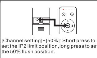
[Channel setting]+[50%]: Short press to set the IP2 limit position, long press to set the 50% flush position.
