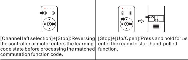
[Channel left selection]+[Stop]: Reversing the controller or motor enters the learning code state before processing the matched commutation function code.
