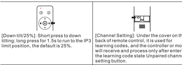
[Down tilt/25%]: Short press to down tilting; long press for 1.5s to run to the IP3 limit position, the default is 25%.
