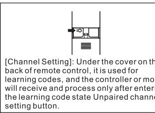
[Channel Setting]: Under the cover on the back of remote control, it is used for learning codes, and the controller or motor will receive and process only after entering the learning code state. Unpaired channel setting button.
