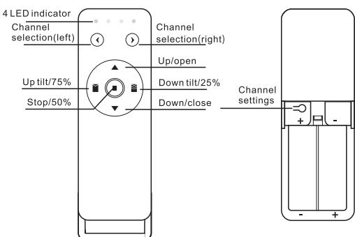
Note: The [channel setting] button is under the cover on the back of remote control.
