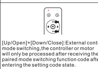
[Up/Open]+[Down/Close]: External control mode switching, the controller or motor will only be processed after receiving the paired mode switching function code after entering the setting code state.
