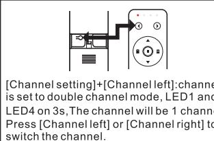
[Channel setting]+[Channel left]: channel is set to double channel mode, LED1 and LED4 on 3s, The channel will be 1 channel. Press [Channel left] or [Channel right] to switch the channel.
