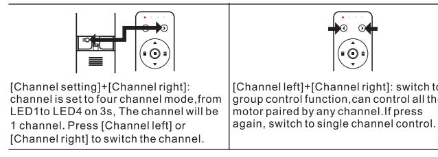
[Channel setting]+[Channel right]: channel is set to four channel mode, from LED1 to LED4 on 3s. The channel will be 1 channel. Press [Channel left] or [Channel right] to switch the channel.
