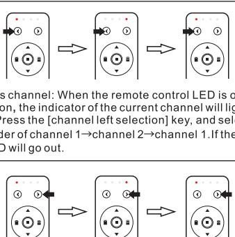
Select the previous channel: When the remote control LED is off, press the [channel left selection] button, the indicator of the current channel will light up, press it again within 3 seconds. Press the [channel left selection] key, and select channels circularly in the order of channel 1→channel 2→channel 1. If there is no operation within 3 seconds, the LED will go out.
