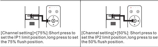
[Channel setting]+[75%]: Short press to set the IP1 limit position, long press to set the 75% flush position.
