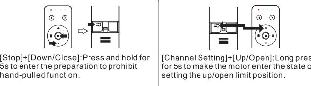
[Stop]+[Down/Close]: Press and hold for 5s to enter the preparation to prohibit hand-pulled function.
