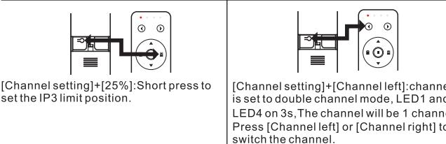
[Channel setting]+[25%]: Short press to set the IP3 limit position.
