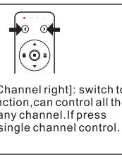
[Channel left]+[Channel right]: switch to group control function, can control all the motor paired by any channel. If press again, switch to single channel control.
