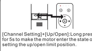
[Channel Setting]+[Up/Open]: Long press for 5s to make the motor enter the state of setting the up/open limit position.
