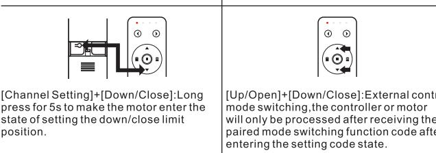
[Channel Setting]+[Down/Close]: Long press for 5s to make the motor enter the state of setting the down/close limit position.
