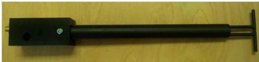
Figure 1 – MVG COMOSAR Validation Dipole
