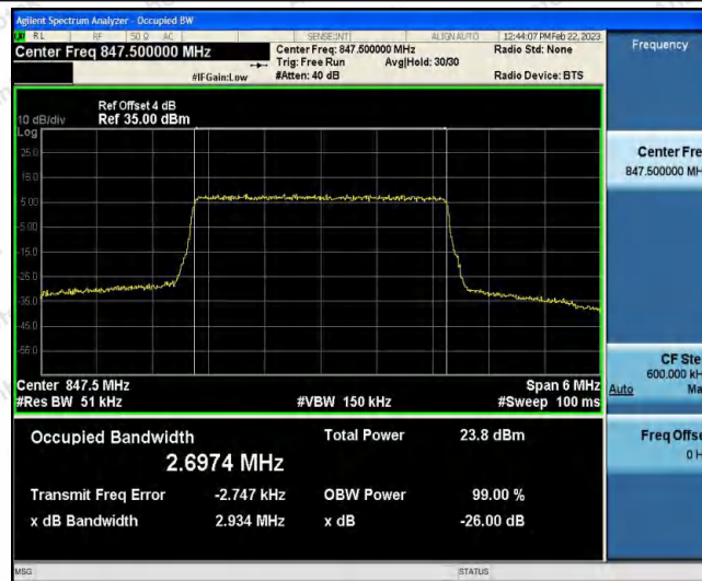
Band5-5MHz-QPSK-20425-25RB#0
