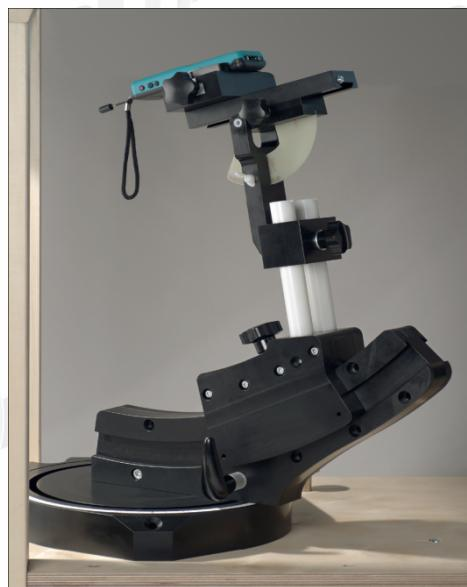
The DASY device holder is designed to cope with different positions given in the standard. It has two scales for the device rotation (with respect to the body axis) and the device inclination (with respect to the line between the ear reference points). The rotation centres for both scales are the ear reference point (ERP). Thus the device needs no repositioning when changing the angles.
